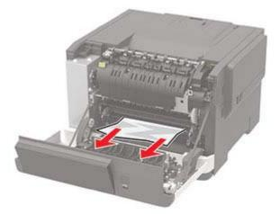
**3** Open the fuser access door, and then remove the jammed paper.
